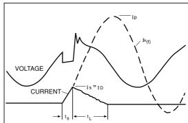
The cut-off current of our h.v. h.b.c. fuse links, which can be taken from the diagram, are a function of the prospective short-circuit current (r.m.s. value of the symmetrical component) and of the rated current.
